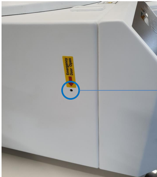
Emergency Door Open Hole
