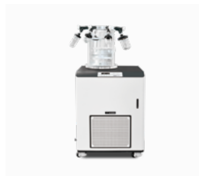
6 Acrylic Chamber with Rubber Valve (8)
