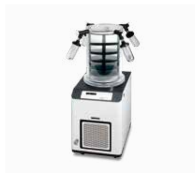
9 Acrylic Chamber with Rubber Valve (4, 8) (Heating)
